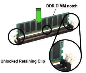
Firmly insert the DIMM into the socket until the retaining clips snap back in place and the DIMM is properly seated.
